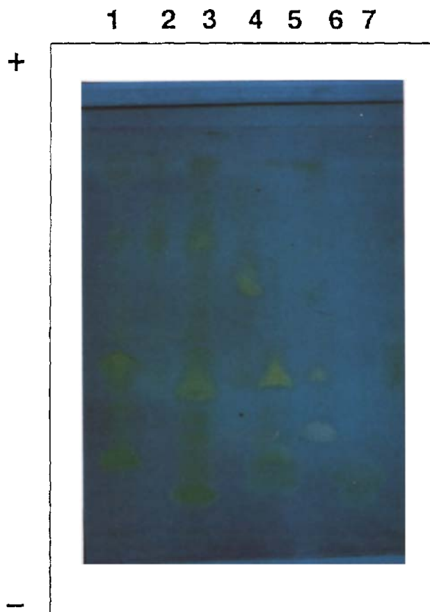
Figure 2. Detection of partially purified P. aeruginosa PA01 siderophores in the CAS overlay after IEF. Estimated total siderophore loading: lane 1, 1.76 nmole siderophores; lane 2, 0.176 nmole siderophores; lane 3, 0.0176 nmole siderophores; pI, pI standards. Anode (+) and cathode (-).
